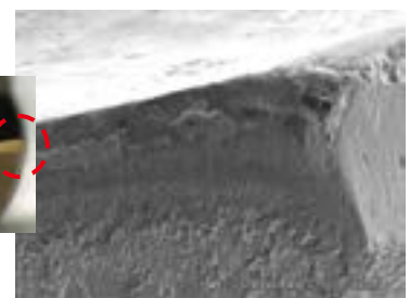
1000穴加工後の刃先 Flute tip after machining 1,000 holes
