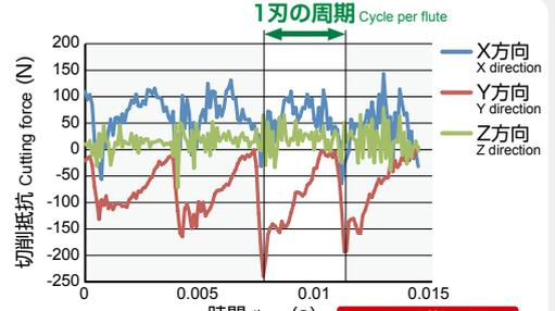
The vibration can be observed a cycle per flute. **振動が確認できる**
