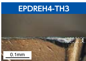
逃げ面摩耗幅 0.029mm Flank wear
