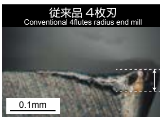
従来品 4枚刃 Conventional 4flutes radius end mill 逃げ面摩耗幅 0.058mm Flank wear
