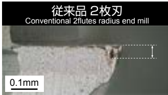
従来品 2枚刃 Conventional 2flutes radius end mill 逃げ面摩耗幅 0.065mm Flank wear
