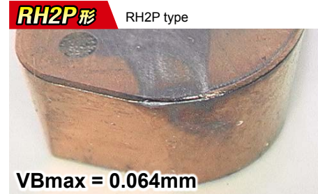
図 60min加工後の工具摩耗状態 Wear condition : after 60 minutes of cutting
