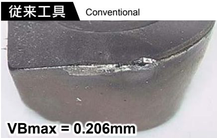
図 60min加工後の工具摩耗状態 Wear condition : after 60 minutes of cutting
