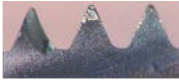
従来品 10穴加工後 Conventional after threading 10 holes.
